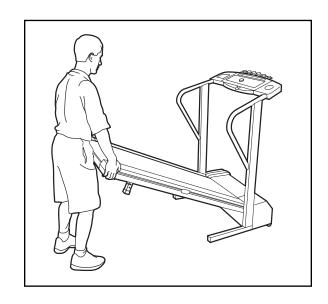
Move your right hand to the position shown at the right, and hold the treadmill firmly. Raise the treadmill until the storage latch locks over the catch. Make sure that the storage latch closes fully over the catch.
